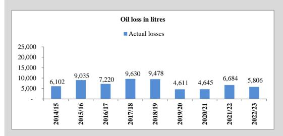
The losses from NGED East Midlands' fluid filled cables can vary from year to year generally dependent on the number of small leaks at disparate locations.
